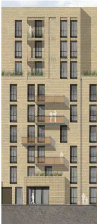
Design Development - Final Proposal Recessed Brickwork Panels
